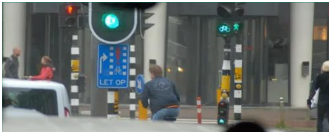
Figure 2.3.3.2: Example from the Netherlands of traffic signals + give way signage controlling turning traffic and cyclists (Source: Dutch Design Guide Ontwerpwijzer Fietsverkeer)
